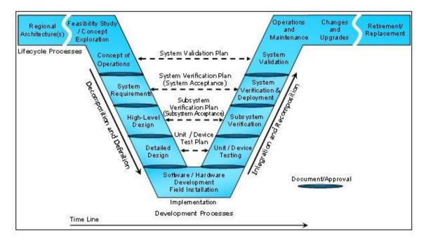
Figure 1. The systems engineering "V" model, depicting the systems engineering life cycle (Federal Highway Administration, 2013).
